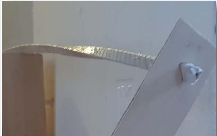
*Figure 4 : Twisting of the triangle beam
