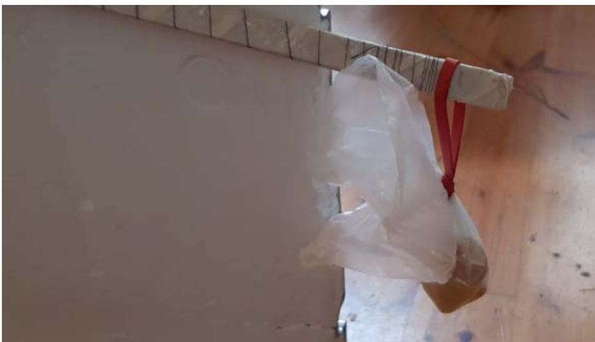
Thereafter I measured the twist, the circular bending of the "rod". I made a simple plywood plate with a triangle hole and put the same weight to measure the twist to clockwise and anticlockwise again in all three positions of the rod resulting in six measures together.
