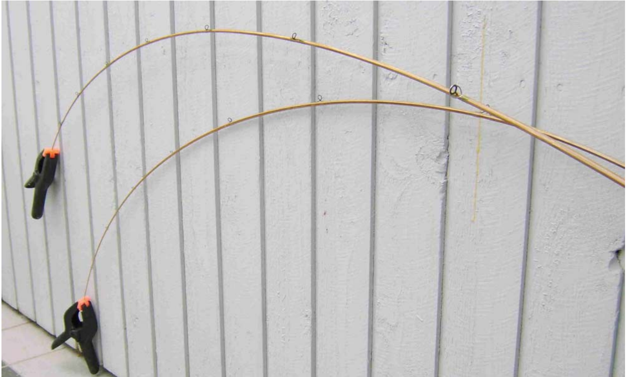
The original #7.4 and modified #3.6 rods in a bending test.
