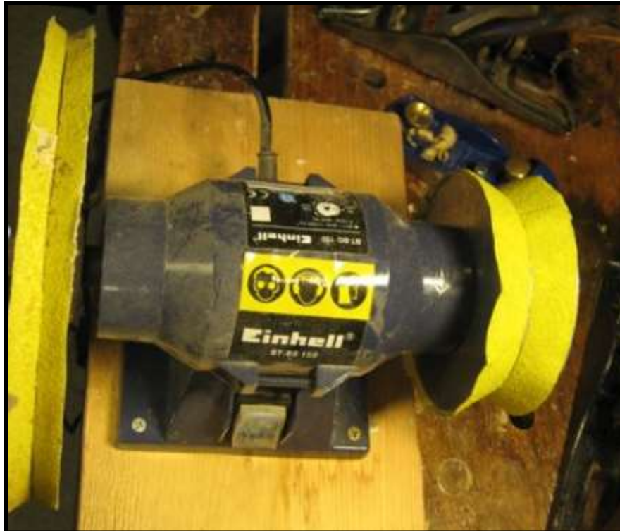
Baginski beveller for 120 degree corners for the triangle rod.
